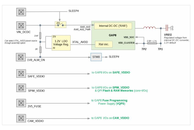
Fig. 3 – On-board power supply generation and control (notional)
